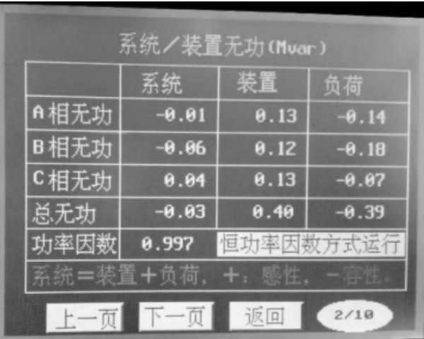
图 8 双向变流装置额定功率下补偿 SVG 数据显示 Fig. 8 SVG data display for compensation under rated power of bidirectional converter device
